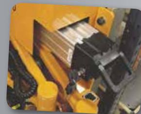
Sky Lifter runs non-stop with extra batteries (optional extra) which are easy to replaced without the need for tools.
