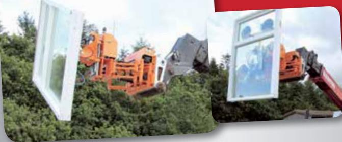
Sky Lifter's smooth pattern of movement is repeated in the yoke where rotation, tilt and tip take place in soft, stepless movements.
