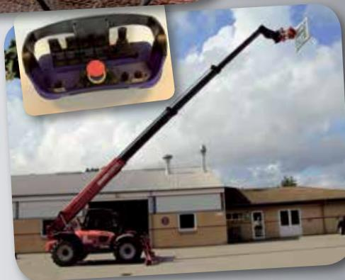
As Sky Lifter is radio-controlled, there are no limits to working height. The range of the remote control is 100 metres.
