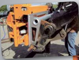
Sky Lifter is easy to install on the telescopic loader using an adapter for Quick release.
